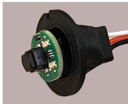
Once the two pieces are separated, the circuit board must be removed from the shell to access the trace cuts on the back of the board. To do this gently push the cable connector into the rear of the shell
