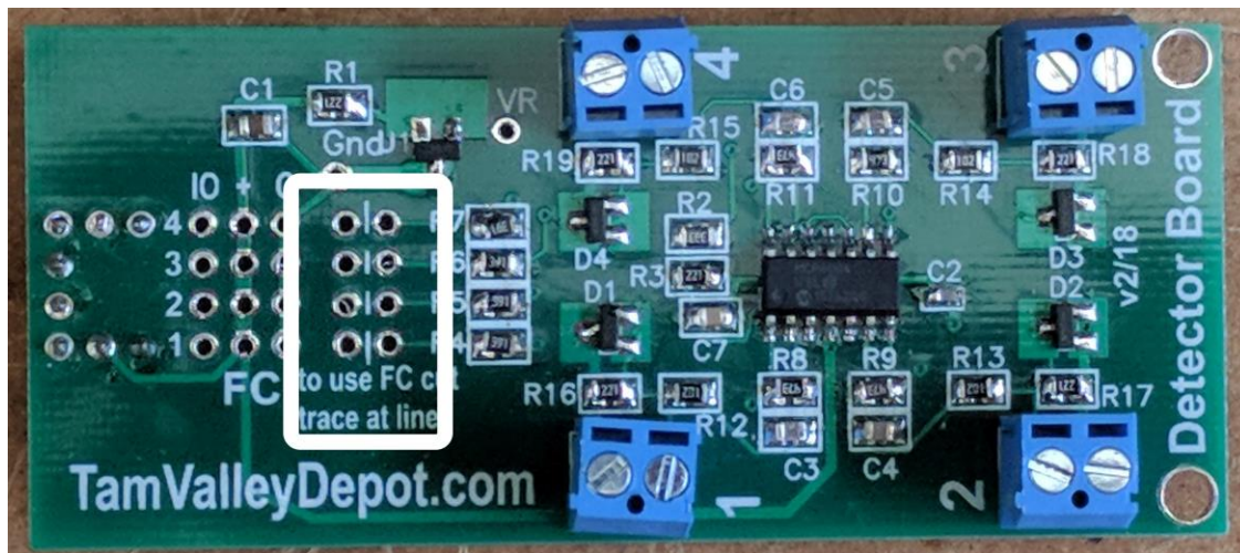
Figure 0-1. Fascia Controller Cuttable Traces
