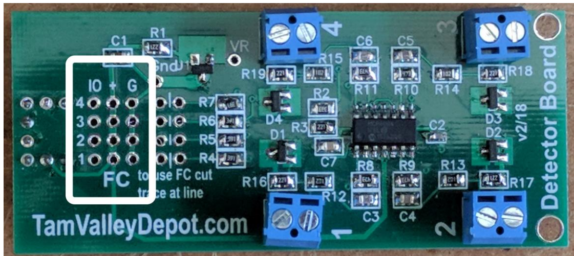
Figure 0-2. Fascia Controller 3-Pin Headers
