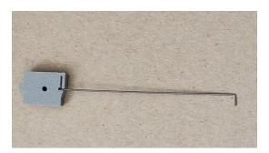
5. With the L-bend of the new wire pointing up and away from the face of the slide, pull the free end of the throw wire until the L-bend aligns with the short channel as shown in the left image. Next press the L-bend into the short channel as shown in the right image. It will probably be a loose fit.
