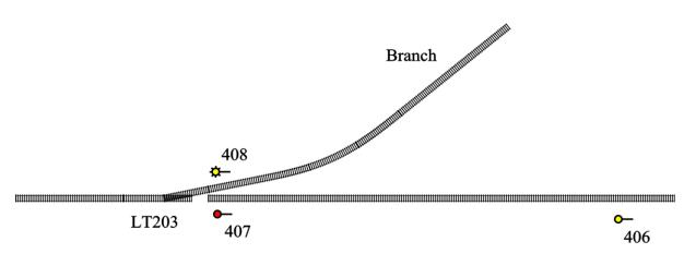
Turnout set to Branch. Signals after delay.
