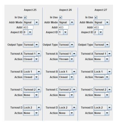
Stop. The first column has Aspect ID set to **0** which is the Stop Aspect. Turnout A Out is set to **Turnout 1**, the *QuadLN\_S* Turnout output that drives the servo that controls the Semaphore. The Action is set so that the blade is horizontal. Turnout B Out is set to **Lock 1**, and the Action is set to **Closed** so that the servo is not forced to the midpoint. The Mode for Turnout C and Turnout D is **None** so they have no effect.
