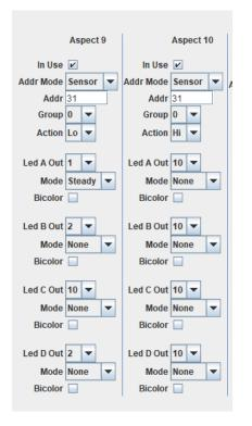
On. The first column has Addr **31** and Action **Steady** which is the Sensor Active (Lo) Aspect. Led A Out is set to the desired Indicator LED. The Mode for Led A is **Steady**. The Mode for the remaining entries is **None** so they have no effect.
