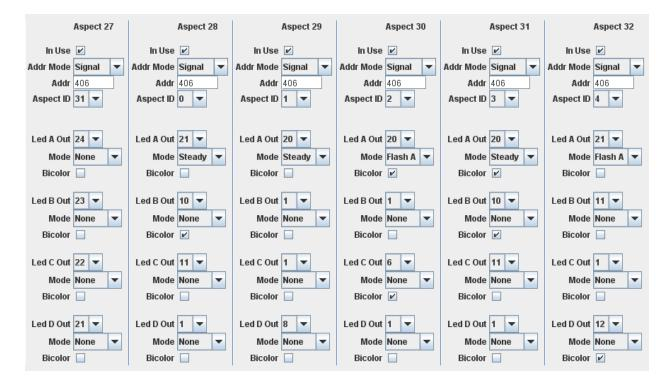
Dark. The first column has Aspect ID set to **31** which is the Dark Aspect. The Mode for all 4 Output entries is set to **None** so that no Outputs are On.
