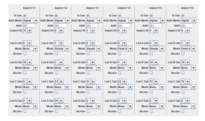
Dark. The first column has Aspect ID set to **31** which is the Dark Aspect. The Mode for all 4 Output entries is set to **None** so that no Outputs are On. The values of the Led Out number and Bicolor checkbox do not matter when the Mode is **None**.
