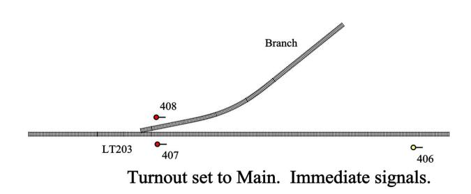
• After a delay, Route 1 sets Signal 407 to Clear and Signal 406 to Clear.
