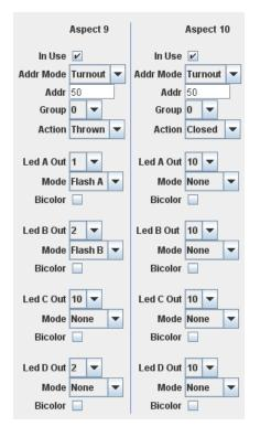
Flash. The first column has Addr **50** and Action **Thrown** which is the Flash Aspect. Led A Out is set to one of the crossing LEDs. The Mode for Led A is **Flash A**. Led B Out is set to the other crossing LED. The Mode for Led B is **Flash B**. This causes the two LEDs to flash alternately. The Mode for the remaining entries is **None** so they have no effect.
