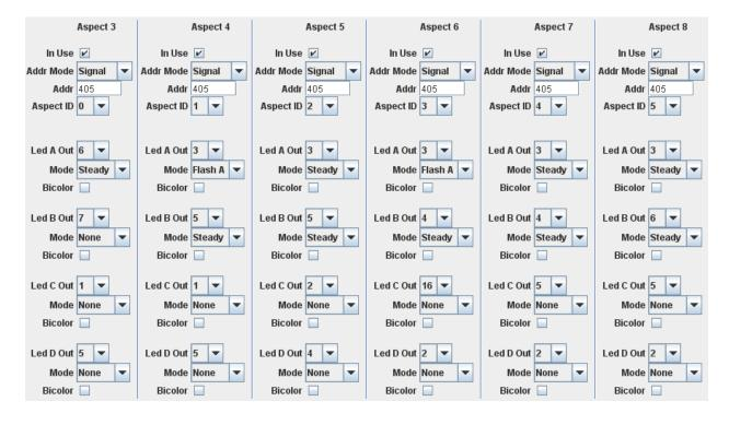
Stop. The first column has Aspect ID set to **0** which is the Stop Aspect. Led A Out is set to the horizontal LEDs. The Mode for the remaining entries is **None** so they have no effect.
