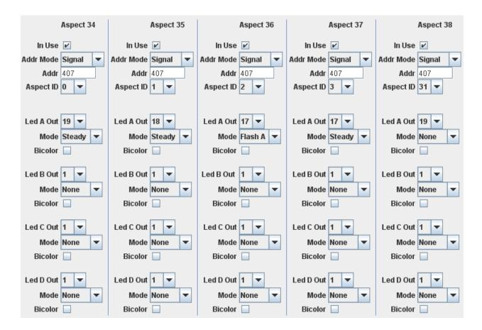
Stop. The first column has Aspect ID set to **0** which is the Stop Aspect. Led A Out is set to the Red LED. The Mode for Led A is set to **Steady**. The Mode for the remaining Output entries is set to **None** so they have no effect.
