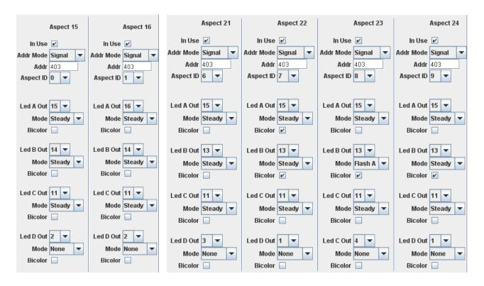
Stop. The first column has Aspect ID set to **0** which is the Stop Aspect. Led A Out is set to the top head Red LED. Led B Out is set to the middle head Red LED. Led C Out is set to the lower head Red LED.
